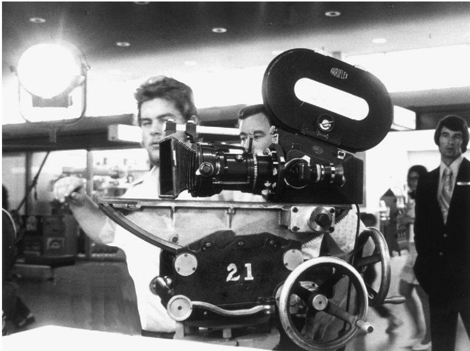
Figure 2.2 I'm standing just behind the lens of a 16 mm Arriflex sitting atop the giant 100 Moey gear head specially designed for the giant MGM 65 mm cameras. This particular gear head was one of the set used in William Wyler's Ben-Hur . Photo by David Yewdall.
